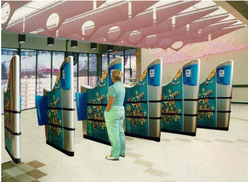
Fig 1 - Using RFID techniques to scan a cart or basket full of groceries in a few seconds; its features include: a scanner to detect and identify the tag attached to each item; electronic payment with smart cards or magnetic swipe cards.
