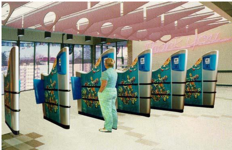
Fig 1 - Using RFID techniques to scan a cart or basket full of groceries in a few seconds; its features include: a scanner to detect and identify the tag attached to each item; electronic payment with smart cards or magnetic swipe cards.
